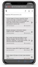
XRD searches for the matching TIPS document based on symptoms and fault codes. After selecting a document, you are automatically forwarded to XENTRY Tips mobile.
