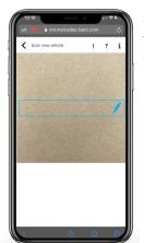
Scan a FIN/VIN with XRD to start the diagnosis process.
